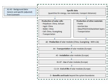
The PolySi, ingots, wafers, cells and modules are manufactured in China. The supply chain is shown below:
