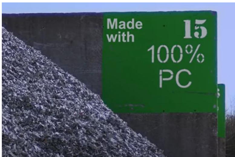
Figure 2: Shredded and sorted post-consumer scrap ready for remelting into new CIRCAL 100R extrusion ingots.
