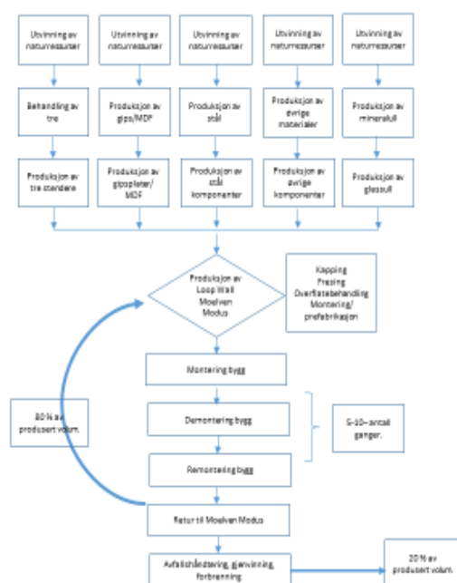
Figure 1. Flow diagram for the production of Loop Wall 400 - MDF system.
