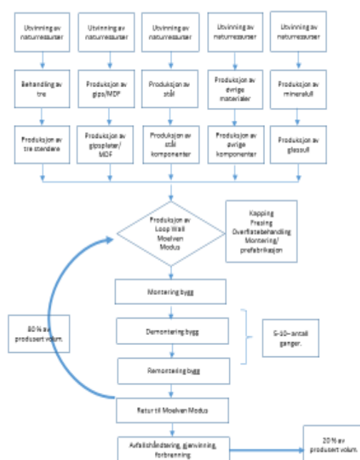
Figure 1. Flow diagram for the production of Loop Wall 300 - Gypsum system.
